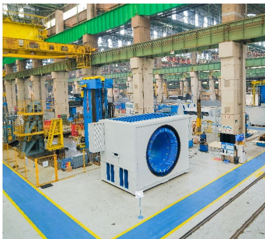
Synchronous condenser manufacturing at ANDRITZ in Araraquara (São Paulo) Copyright: ANDRITZ
